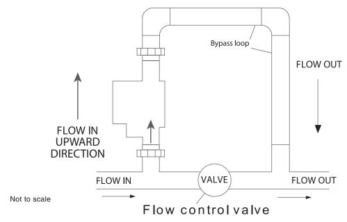
iChlor SCG System Loop Plumbing Diagram
