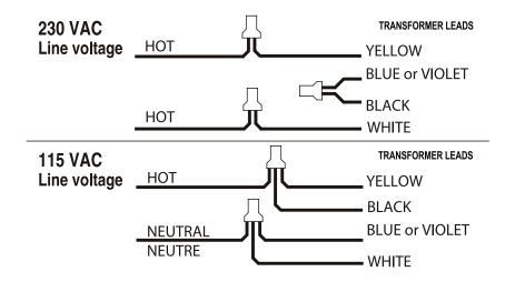
iChlor Power Center 230 and 115 VAC Transformer Wiring
