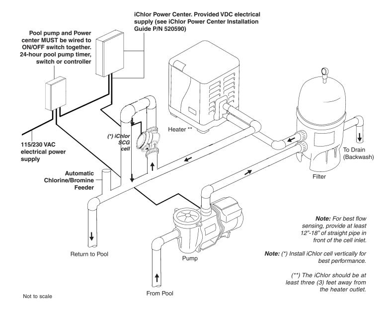
iChlor System Schematic Diagram
