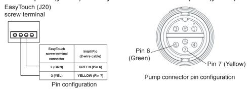
Insert the screw terminal onto the EasyTouch COMPORT (J20) board connector.
